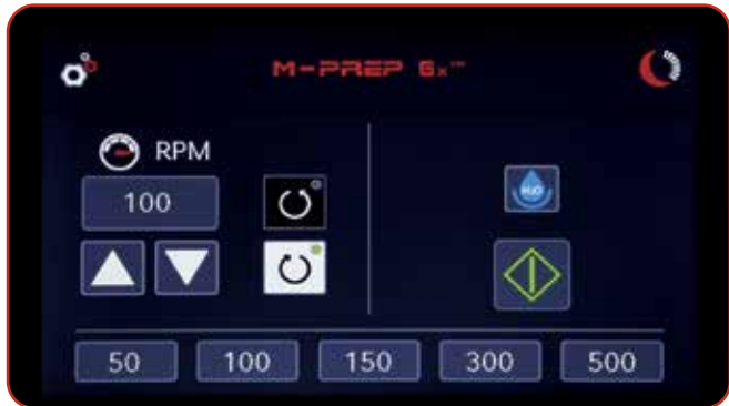
The 7" color LCD touchscreen is used to control all functions and is extremely easy to navigate, allowing greater efficiency among users.
